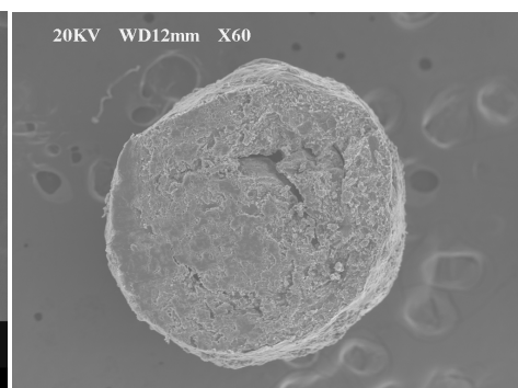
Fig. 6: SEM of transverse section of polymer coated NPS.
