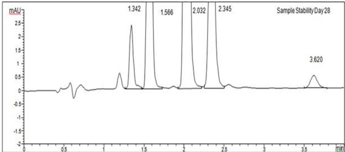
Fig. 8B: Chromatograms of naturally aged API and impurity samples: Day 28.
