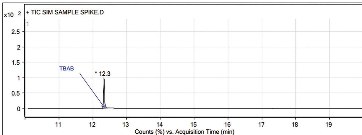
**Figure 3.** GC-MS chromatogram of Teneigliptin spiked with TBAB.
