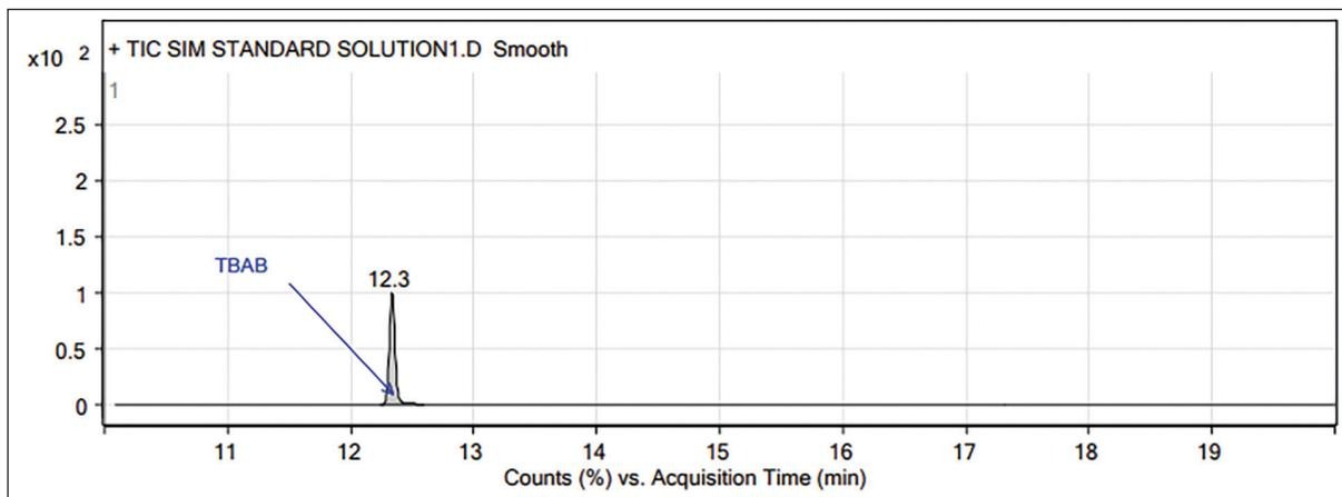
**Figure 1.** GC-MS chromatogram of TBAB standard (1,000 ppm).
