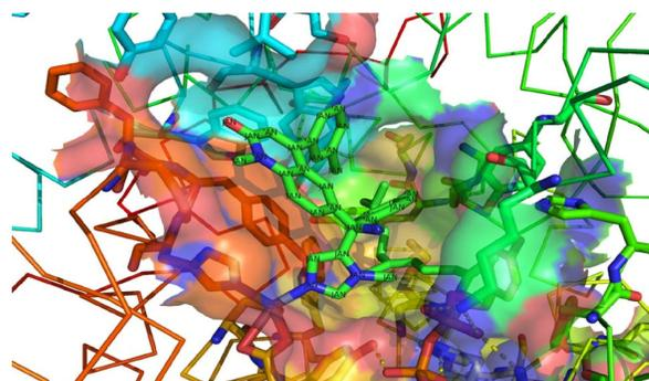
**Fig 3:** Tipifarnib (green) docked in the active site cleft between the 2 subunits of Ftas covalently bound with Zn (II).
