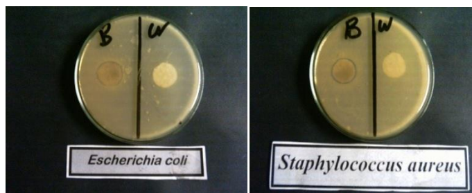
Fig. 9: Antibacterial Activity of treated and untreated samples. Where, w) untreated fabrics and B) treated fabrics.
