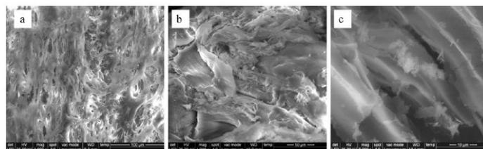
Fig.1: Scanning electron micrographs of pullulan (a), and copolymerized pullulan with different grafting ratio: 29% (b) and 41% (c). (Source: Marieta et al, 2011)
