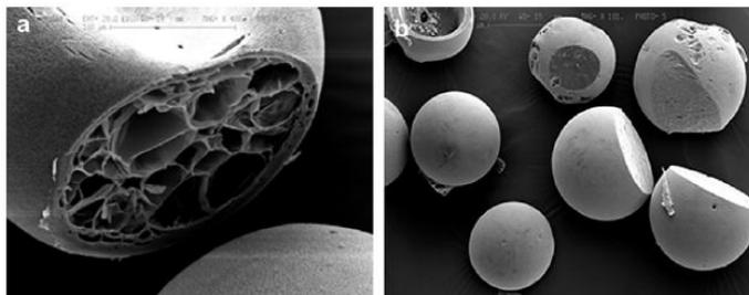
**Fig.2:** Scanning electron micrographs of pH and temperature sensitive pullulan microspheres prepared before (a) and after (b) grafting. (Source: Gheorghe et al, 2008).
