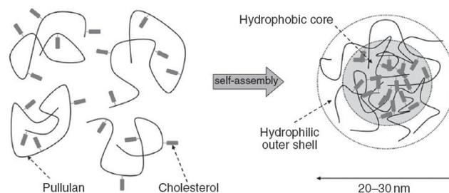
**Fig.3:** Formation of cholesteryl-pullulan conjugate-based nanoparticles by self-aggregation in aqueous solution (Source: Lee et al, 2004).
