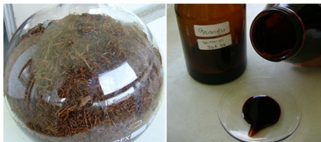
Fig. 1: The tobacco leaves macerated with 95% ethanol in round bottom flask (Left) and an appearance of the tobacco extract (Right).
