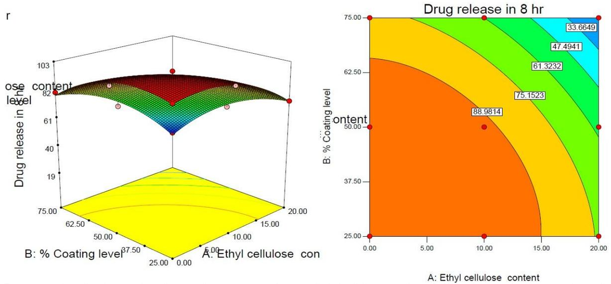
**Fig. 3:** Response surface plot showing the influence of percentage weight ratio of ethyl cellulose to eudragit L 100 and coating level on cumulative drug release at 8 hr and corresponding contour plot showing the relationship between various levels of 2 critical process parameters (CPPs).
