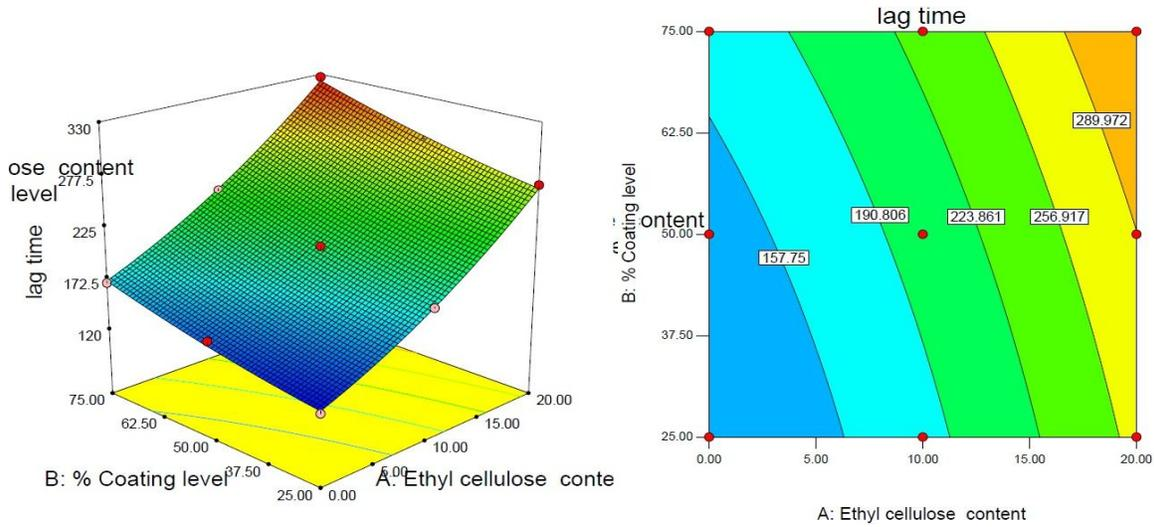
**Fig. 2:** Response surface plot showing the influence of percentage weight ratio of ethyl cellulose to eudragit L 100 and coating level on lag time and corresponding contour plot showing the relationship between various levels of 2 critical process parameters (CPPs).
