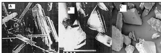
Fig. 3: Scanning electronic micrograph of a) pure drug, b) Eudragit E-100 and c) SDS formulation.
