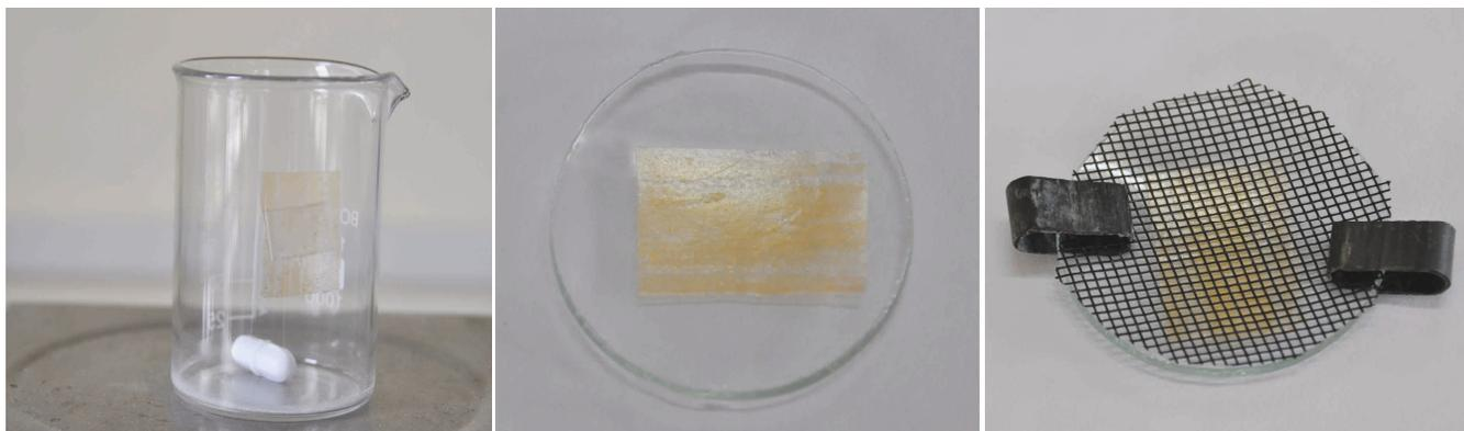
**Fig. 1:** Dissolution setups for Method I (beaker stirrer method) and Method II (Apparatus 5 method).
