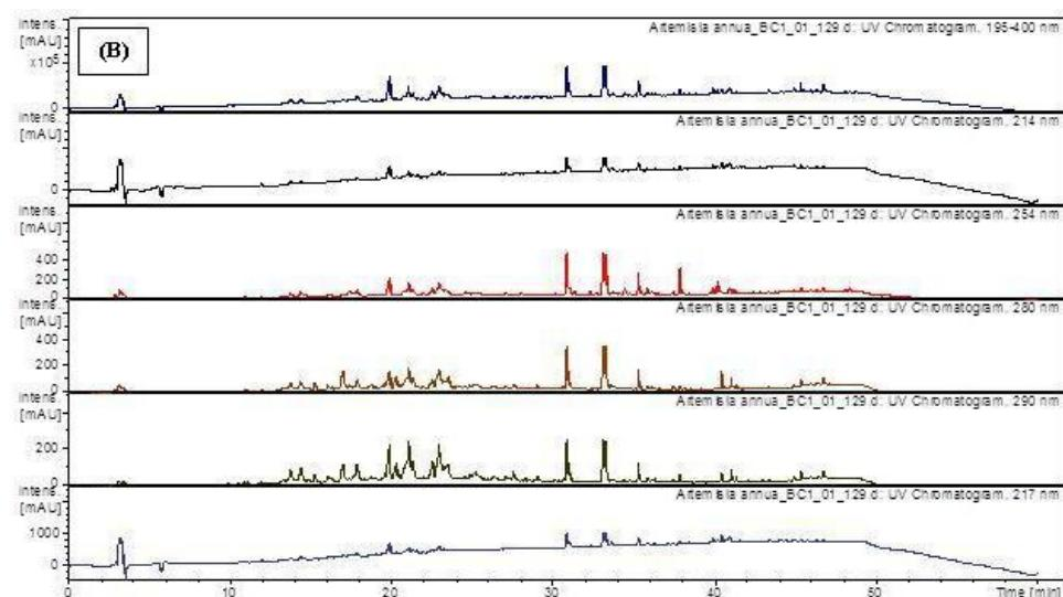
**Fig. 1(B):** Typical HPLC-DAD chromatogram of the crude methanolic extract of *Artemisia annua* monitored at 214, 217, 290 and 280 nm and UV spectra (DAD) recorded between 195 and 500 nm showing very low absorbance of artemisinin peak in the ultraviolet (UV) regions compared with the LC-positive mode ESI-MSn base peak chromatogram (BPC) profile.
