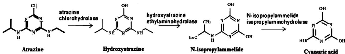
**Fig. 7:** Proposed degradation pathway of atrazine by *Pichia kudriavzevii* Atz-EN-01.
