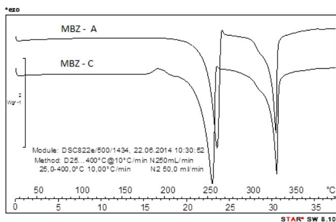
Fig. 8: DSC curves for samples of MBZ raw material A and polymorph C.
