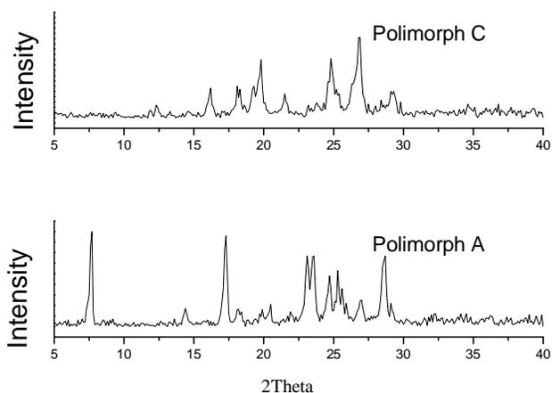
Fig. 6: Diffractogram of the sample MBZ polymorph C and A.
