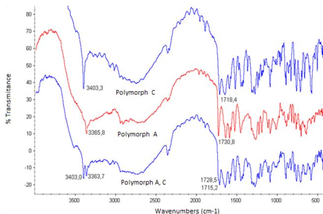
Fig. 7: Infrared spectrum for samples of MBZ form A and C.
