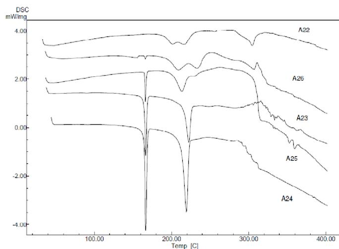
Fig. 10: DSC curves for samples of MBZ tablet.
