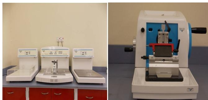
Fig. 2: (A) Tissue Embedding Center (TEC 2900) (B) Rotary Microtome (Histo Line Laboratories Brand).
