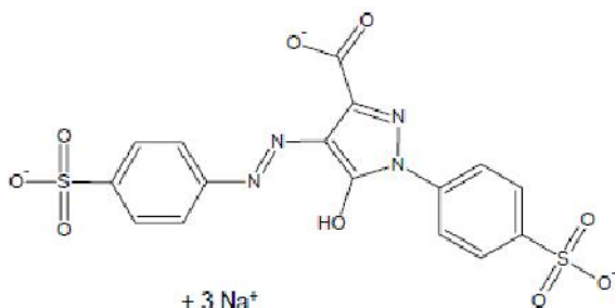
Fig. 1: Chemical structure of Tartrazine (trisodium salt of 3-carboxy-5-hydroxy- 1-(p-sulphophenyl)-4-(p sulphophenylazo) pyrazole.
